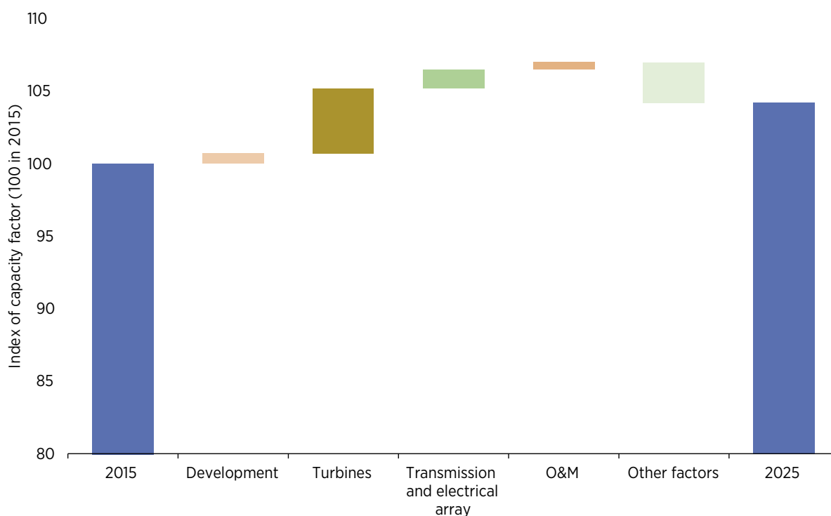
FIGURE 36: PROJECTED IMPROVEMENT IN ELECTRICITY YIELD AT OFFSHORE WIND FARMS FOR THE SAME QUALITY WIND RESOURCE, 2015 AND 2025
